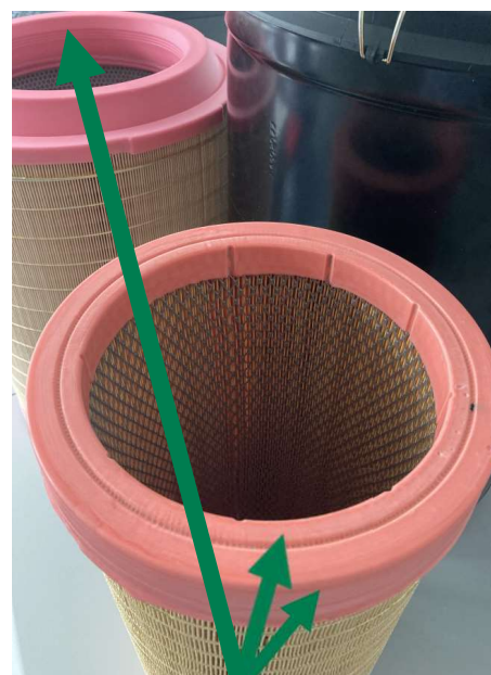
cover secondary element and inner side main element should be greased
