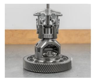
• The tapered roller bearing on the gearbox side of the equalising gearbox
