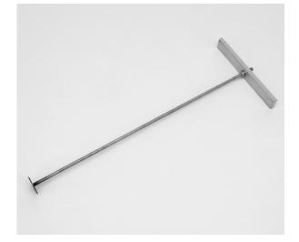
• Insert the lifting device with the output shaft in the housing
