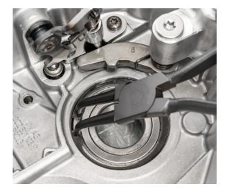
• Press the ball bearing of the input shaft out of the gearbox housing
