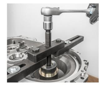
• Press in a new shaft seal ring on the motor side of the differential gearbox
