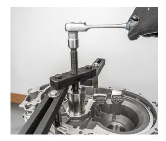
• Press in the new motor-side bearing outer ring of the output shaft again
