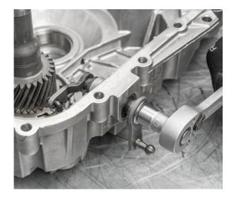
• Remove the shaft seal of the selector shaft using a suitable tool
