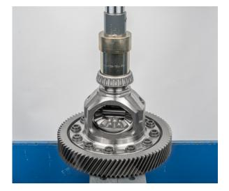
• Press off the tapered roller bearing on the motor side of the output shaft
