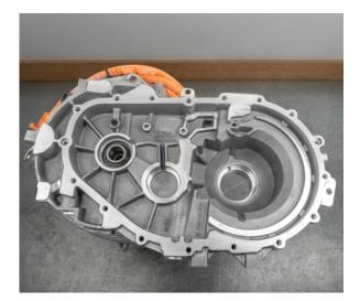
• Remove the shaft seal of the rotor shaft
