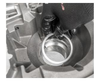
• Press in the new motor-side bearing outer ring of the differential again
