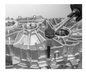
• Fitting the drive shaft circlip
