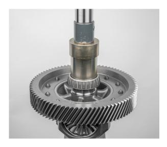
• Press the new motor-side tapered roller bearing onto the differential gearbox
