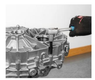
• Lift the gearbox housing evenly upwards using a suitable tool (e.g. mounting lever)
