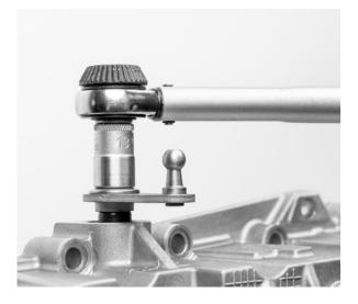
• Press the input shaft out of the gearbox housing
