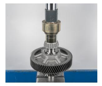
• Press the new motor-side tapered roller bearing onto the output shaft
