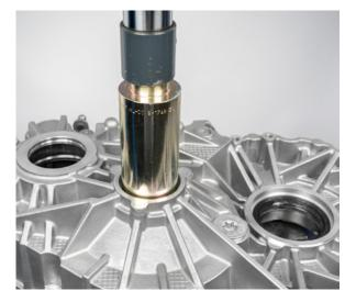
• Remove the shaft seal ring on the gearbox side of the differential
