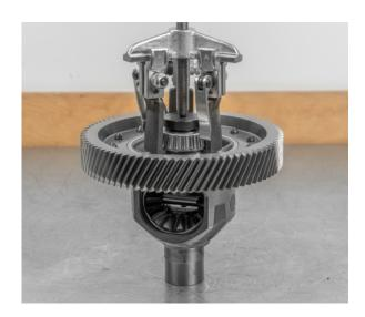
• Press a new tapered roller bearing on the gearbox side onto the differential gear
