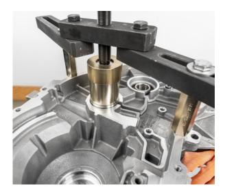
• Press in new motor-side bearing outer ring of the differential **without** adjusting disc
