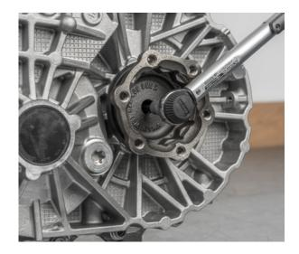
• Replace the sealing ring of the gearbox housing breather
