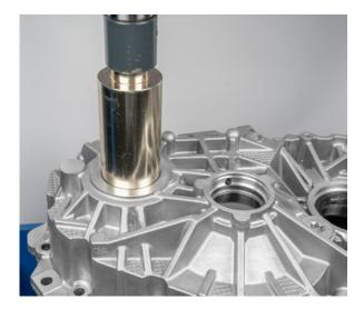
• Press out the bearing outer ring of the output shaft from the gearbox housing
