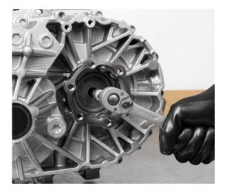
• Remove the shaft seal ring on the engine side of the drive shaft flange
