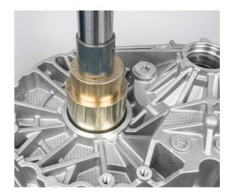
• Press the new ball bearing of the input shaft into the gearbox housing
