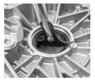
• Remove the bearing outer ring on the gearbox side using a suitable internal extractor
