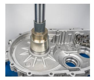
• Press a new shaft seal ring on the gearbox side of the differential into the gearbox housing
