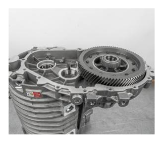
• In order to measure the axial play of the output shaft, a suitable lifting device such as a threaded rod with a welded-on shim is required
