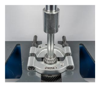
• Press a new tapered roller bearing on the gearbox side onto the output shaft
