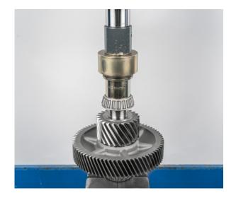
• Insert equalising gear in the housing
