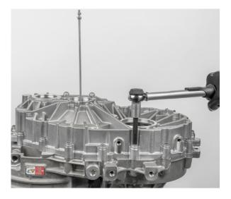
• To determine the differential setting disc, mount the dial gauge as shown and ensure that the measuring tip is preloaded
