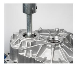
• Remove the retaining ring of the input shaft bearing
