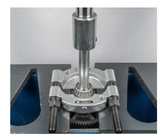
• Press off the tapered roller bearing on the gearbox side of the output shaft
