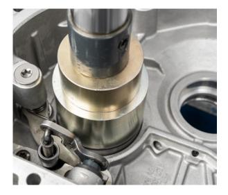
• Fitting the circlip
