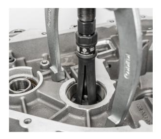
• Insert the previously determined adjusting disc (e.g. 1.35 mm) into the bearing seat
