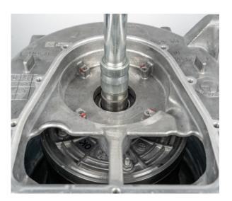
• Disassemble the snap ring inside the housing.
