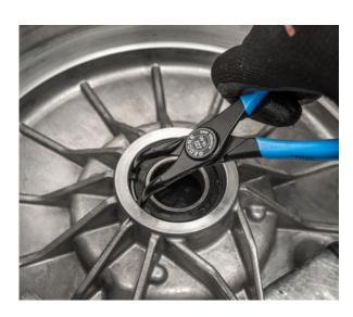
• Press the bearing out of the housing.
