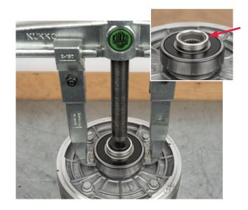
• Press on a new ball bearing.
