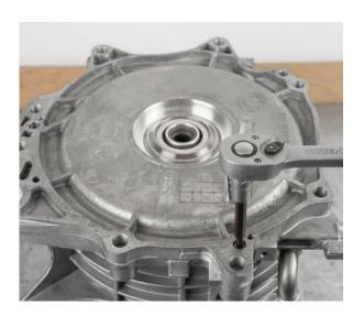
• Remove the rotor from the stator housing.
