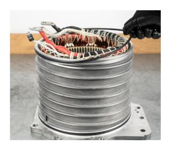
• Assemble the new O-rings and lubricate them using suitable grease, e.g. BMW assembly grease GE.
