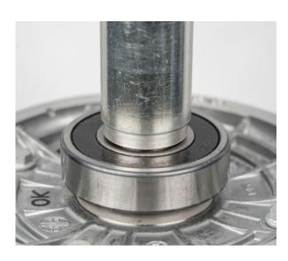
• Press the bearing onto the rotor along with the housing.
