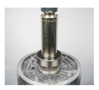
• Press on the contact ring to the previous installation depth using a suitable sleeve.
