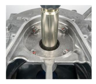
• Press in a new ball bearing.
