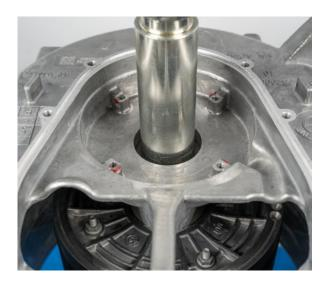
• Check the seat of the spring washer in the bearing seat of the stator housing.
