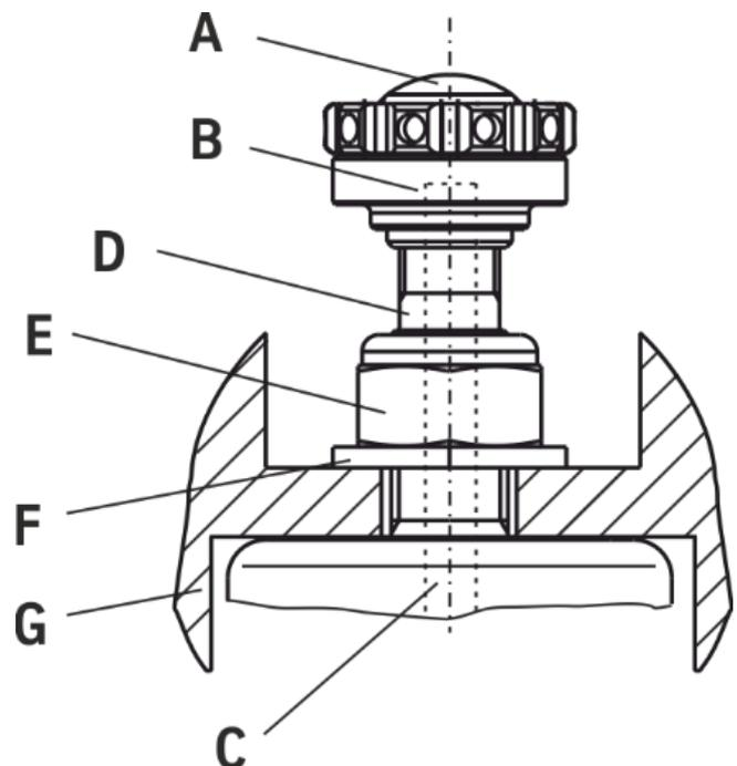
Fit piston rod nut (E) and disc (F) to BILSTEIN strut.
