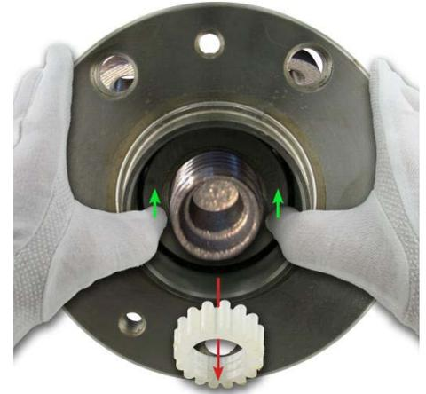
The plastic joining sleeve ring will be automatically pushed out by the axle stub, when mounting the bearing in a correct way, applying the force on the inner ring. Do not push out the plastic sleeve manually before mounting.
