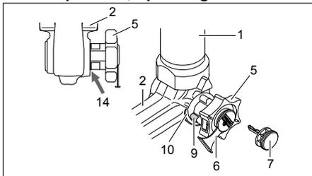
**Unlocked position, ball bar not mounted**
