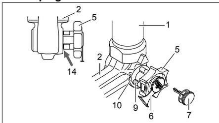
**Position déverrouillée, accouplement non monté**
