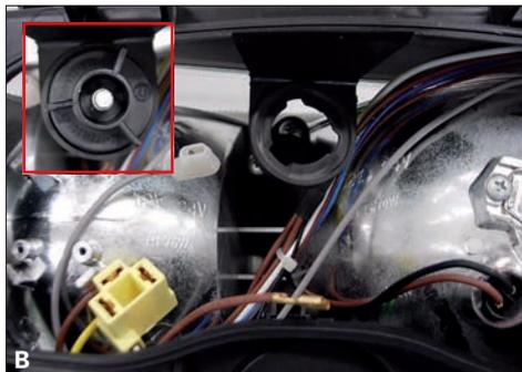
Rotate the reflector bracket clockwise for opening.
