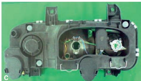
Install the motor and the specified bulb.
