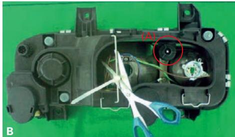
Take out the reflector bracket (A), then use the tool to cut the cable tie and take off the cable tie and spring.
