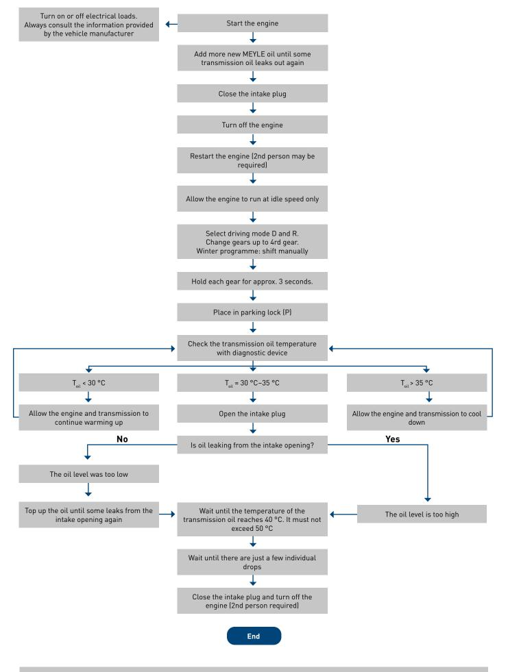
NB: Depending on the type of transmission, it may have a bypass valve which opens or closes the oil circuit to the oil cooler, which is why the drive should be sufficient to ensure the transmission oil temperature reaches at least 75 °C. After the drive, allow the transmission to cool down, check the oil level again and correct if necessary.
