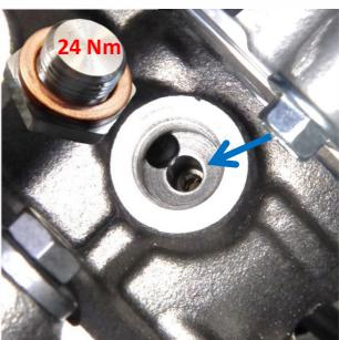
The locking screw is to be tightened with 24 Nm. Never use liquid sealants.
