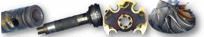
Wear and oil coking on radial bearing
