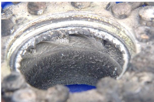
Lime deposits and rust in the VTG unit
