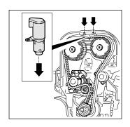
In order to ensure that the new camshaft phasing units operate correctly, the control valves included in the INA Engine KIT must be used.
