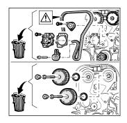
The timing belt must be removed in order to replace the faulty camshaft phasing units. As the timing belt must be replaced at defined intervals, for economic purposes it usually makes sense to also replace the complete timing belt drive together with the tensioner pulley, the deflection pulley and the water pump. In the event of oil leakage, the timing belt drive must be replaced!
