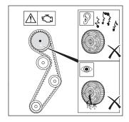
The control valve filter is clogged due to dirt and abrasion. As a result, the camshaft phasing unit is not supplied with sufficient engine oil and is irreparably damaged. This damage is evident in the form of significant noise generation and/or oil leakage.
