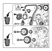
The timing belt must be removed in order to replace the faulty camshaft phasing units. As the timing belt must be replaced at defined intervals, for economic purposes it usually makes sense to also replace the complete timing belt drive together with the tensioner pulley, the deflection pulley and the water pump. In the event of oil leakage, the timing belt drive must be replaced!
