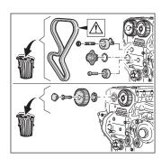
The timing belt must be removed in order to replace the faulty camshaft phasing unit. As the timing belt must be replaced at defined intervals, for economic purposes it usually makes sense to also replace the complete timing belt drive together with the tensioner pulley, the deflection pulley and the water pump. In the event of oil leakage, the timing belt drive must be replaced!
