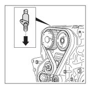
In order to ensure that the new camshaft phasing unit operates correctly, the control valve included in the INA Engine KIT must be used.
