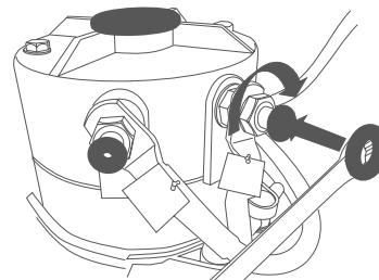
**3.9** Connect the power supply/negative battery lead to the battery. Before starting the system, make sure that the battery is fully charged. Check that the entire electrical system is working properly according to the machine or system manufacturer's instructions.
