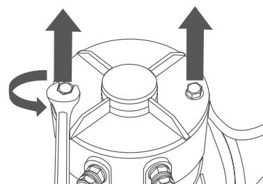
**3.4** Make sure that the motor you are about to install matches the motor you just removed. Using the catalogue, check the electrical part number, the direction of rotation, the rated voltage, the rated current, the fitting dimensions, the electrical connections, etc.
