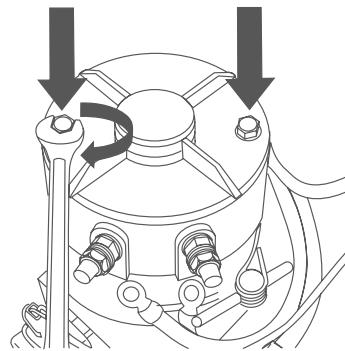
**3.8** Connect the electrical cables to the electric motor. Take care to route the cables properly, making sure that the cables do not come into contact with hot or abrasive surfaces.
