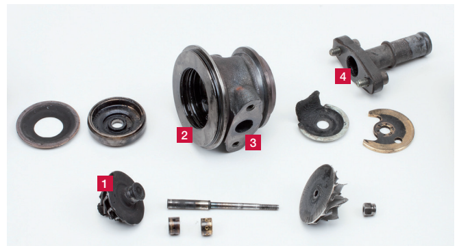
Figure 1: When the DPF is saturated, exhaust gases flow through the turbocharger: from the turbine wheel (1) into the bearing housing (2) and through the oil drain (3) into the return line (4)
