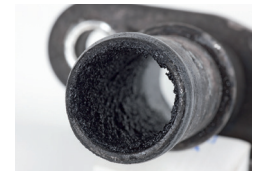
Figure 3: Coked oil return line as a result of exhaust gas penetration
