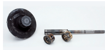
Figure 2: Broken rotor shaft due to inadequate lubrication of the radial bearings
